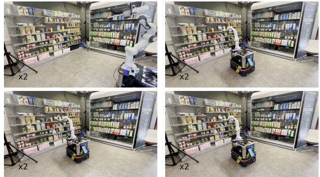
Fig. 7: Trajectory generation with optimization fabrics for mobile manipulator using visual serving for product picking.
