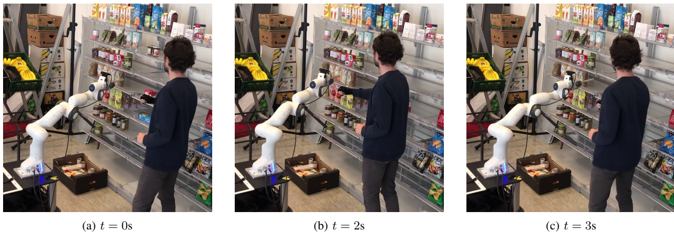
Fig. 5: Dynamic Fabrics in the presence of a human. The human hand’s state is estimated with a motion capture system. The robot smoothly and in advance avoids the human operator and allows for safe coexistence.
