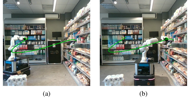
Fig. 1: Dynamic fabrics for path (green) following with a non-holonomic mobile manipulator. Dynamic fabrics control all actuators simultaneously to follow the end-effector path while keeping a given orientation and avoiding collision with the environment.
